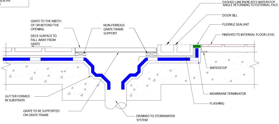
MEMBRANE TERMINATION AT WALL OPENINGS WHERE THE INTERNAL AND EXTERNAL FINISHED FLOOR LEVELS DO NOT ALLOW THE UPTURN (REQUIRED IN AS 4654.2 - 2012, APPENDIX A, TABLE A1)
