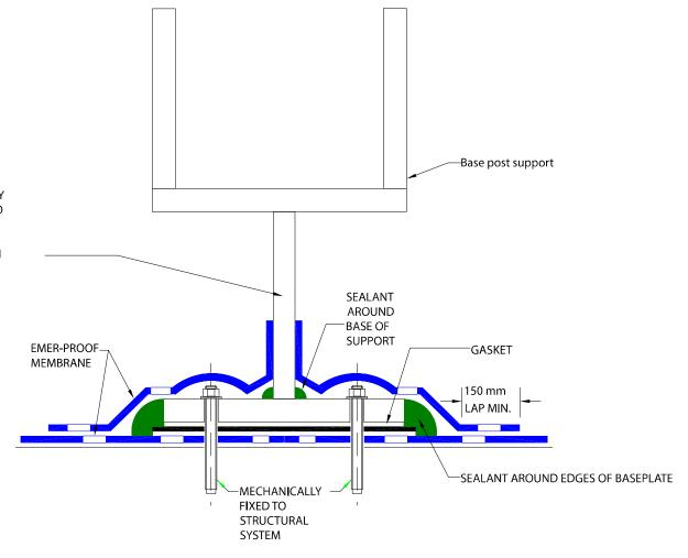
DETAIL OF METAL POST SUPPORT - (b) POST MEMBRANE INSTALLATION
