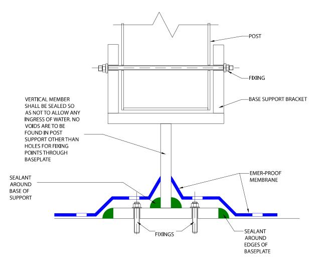
DETAIL OF METAL POST SUPPORT - (a) PRIOR TO MEMBRANE INSTALLATION
