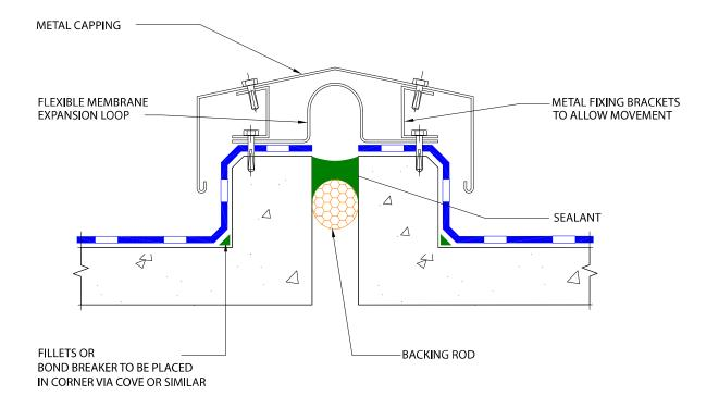
ONE-WAY MOVEMENT JOINT DETAIL
