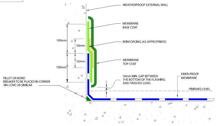
(b) OVERFLASHING CONSTRUCTED OF A LIQUID-APPLIED MEMBRANE
