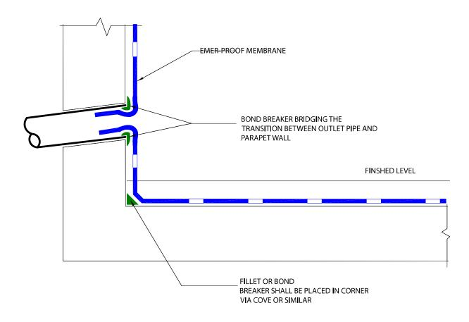
OVERFLOW PIPE THROUGH PARAPET DETAIL
