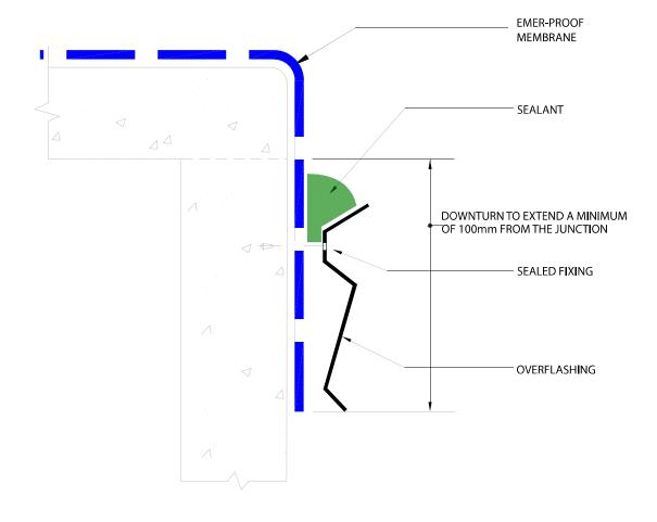
VERTICAL DOWNWARD TERMINATION (b) PRESSURE SEAL
