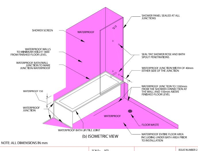
EXTENT OF TREATMENT OF WET AREAS - EXCEEDS AS3740 (CEMENT & COMPRESSED FC SHEET FLOOR)
