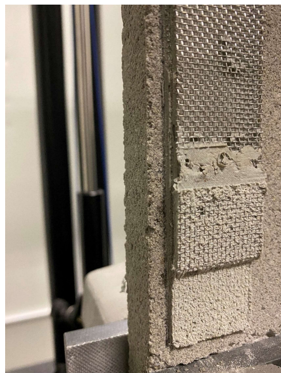
FIGURE 4 IMAGES OF TEST SAMPLE PERFORMING ADHESION-IN-PEEL
