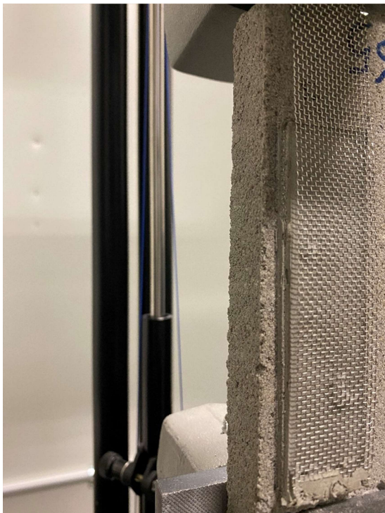
FIGURE 4 IMAGES OF TEST SAMPLE PERFORMING ADHESION-IN-PEEL
