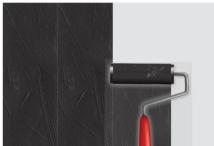
2 Apply the Emer-Clad Facade to the surface in a continuous pattern.
