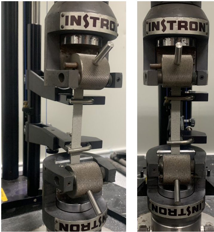
Figure 3 Images of test sample performing durability load / elongation test
